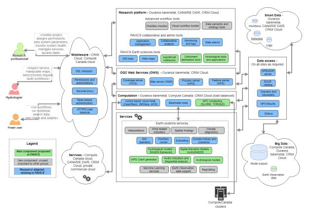
PAVICS nodes are data, compute and index endpoints accessed through the PAVICS platform or external clients. The Node service is the backend that provides data storage, metadata harvesting, indexation and discovery of local and federated data, user authentication and authorization, server registration and management. The *node service* is therefore composed of several services that are briefly described below, accompanied by links to the full documentation of each individual building block.
